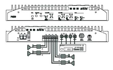
System 2 - P450 used in 2-channel bridged mode with full range speakers.
